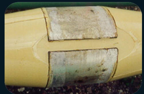
Anode Tapers after FLOMAX FT-6000 elastomer
